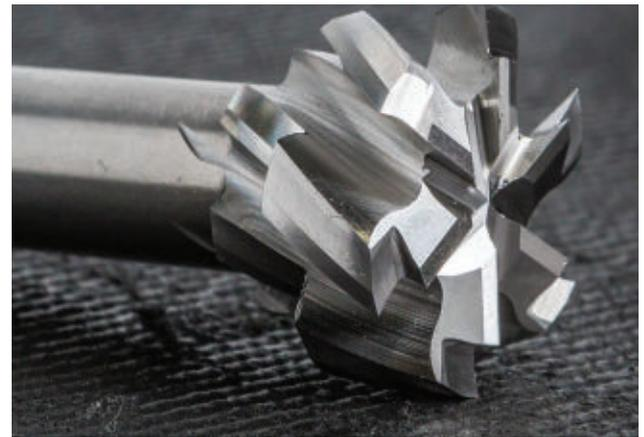
A sample of the grinding performed on the new Walter tool grinder.
