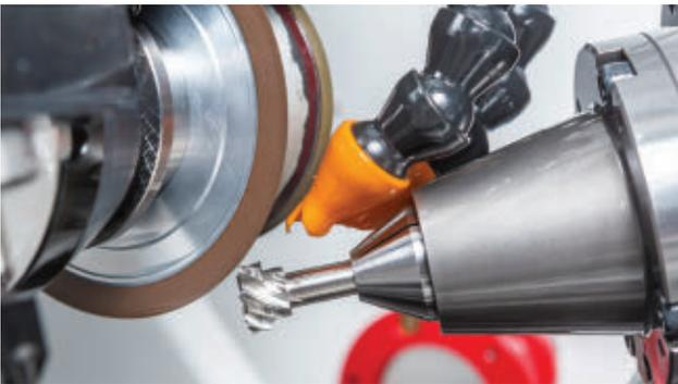
The maximum grinding wheel diameter is 150 mm and grinding speed is 0 to 10,500 rpm.
