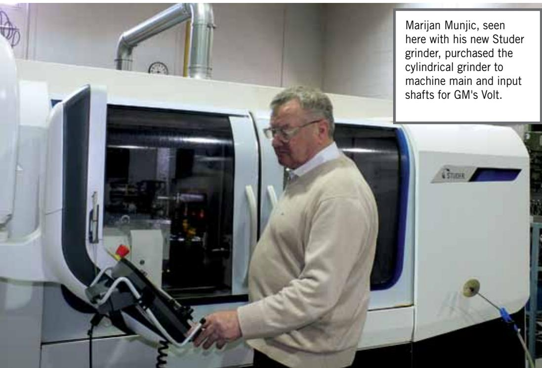
Marijan Munjic, seen here with his new Studer grinder, purchased the cylindrical grinder to machine main and input shafts for GM's Volt.
