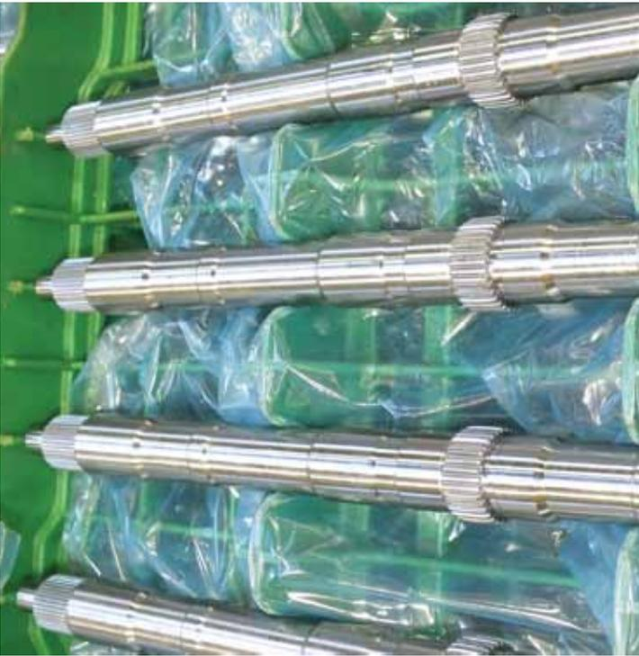
The main shaft is the most critical component of the Volt's electric motor. MTM has also used the Studer to create tight tolerance prototypes for customers.
