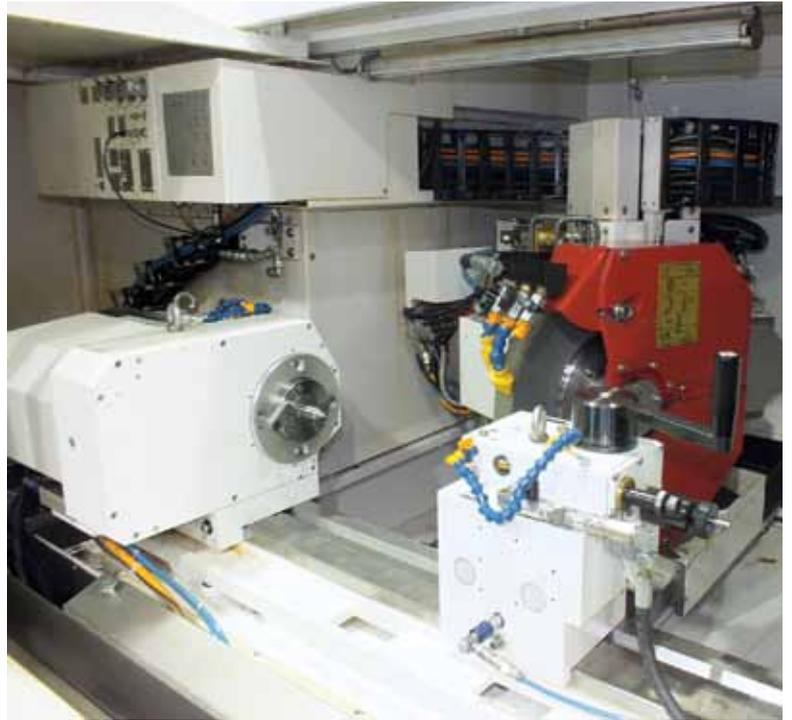
The Studer S33 CNC cylindrical grinder is equipped with a fixed wheelhead with two motor spindles for external grinding and an internal grinding attachment.
