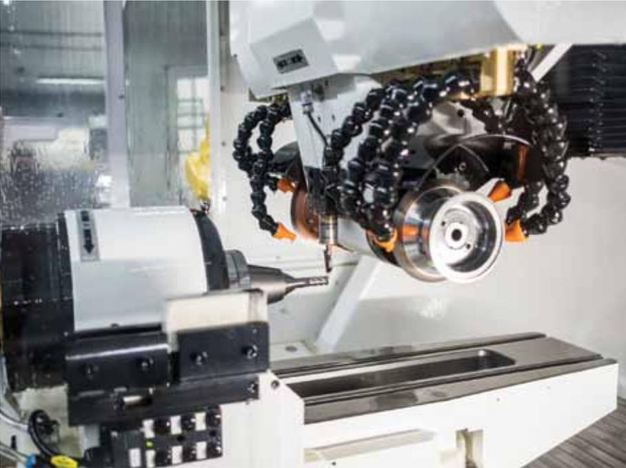
Probing systems from Renishaw pick up tool edges and check for wheel wear.
